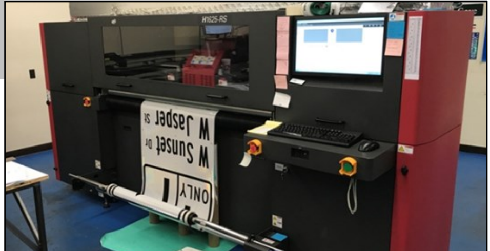
The 3M approved reflective sign digital printer at work in our manufacturing facility in Jackson, Mississippi. It will print up to 48" wide reflective - the widest available - in all of the ASTM approved traffic colors as well as the virtually unlimited spectrum of PMS colors all protected by the 3M Matched Component System warranty.
